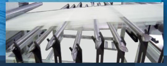
The splitting assembly separates the sized and dried warp yarn into layers for higher production efficiency and better fabric quality.
