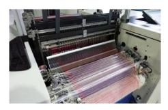
Leno Weave Attachment Available on CCI Sampling Loom Now Leno fabric is ideal for using in new material development for many markets. To cater to the application of leno fabrics in various areas, CCI presents the <u>Evergreen</u> with leno device, which is specifically designed for suiting the complex production of leno weave. Furthermore, equipped with CCI's computer-controlled technology, users are capable of setting different density and weaves more easily.
